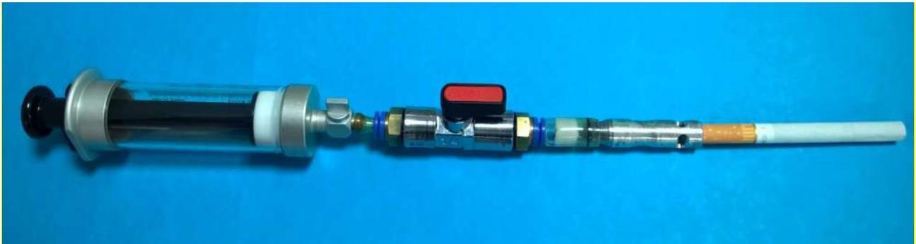
Fig. 2: smoke sampling system
